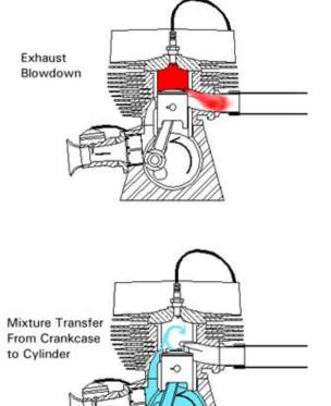
Mixture transfer continues until the piston rises high enough to shut off both the inlet and exhaust transfer ports.
