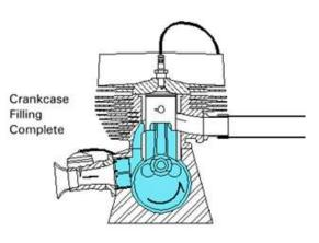
Just as the piston reaches the top of the cylinder, the spark plug ignites the air / fuel mixture (coloured red). Note that THIS MIXTURE WAS PROVIDED BY THE PREVIOUS CYCLE
