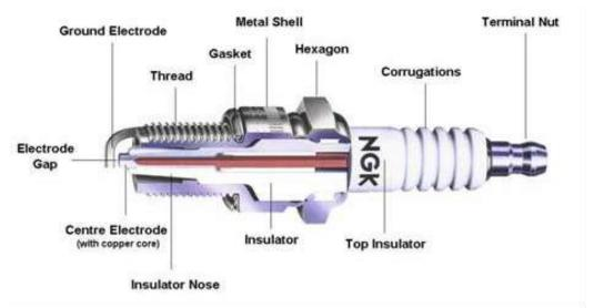
After removal from the engine, the first step is a visual check of the spark plug:
